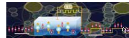
① ② Electric field control of the room-temperature ferromagnetism in the p-type a-CFTBO magnetic semiconductor originating from a ferromagnetic metallic glass
